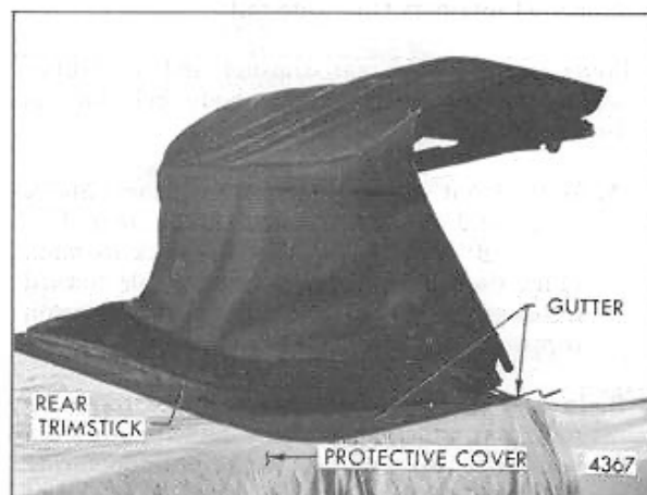
Fig. 9-Rear Trimstick on Rear Deck of Car
