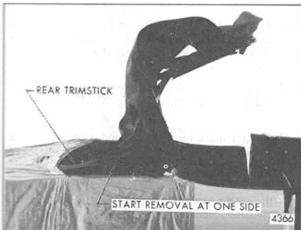
Fig. 8-Lifting Rear Trimstick From Body
